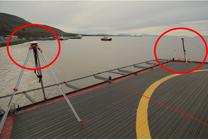
Fig. 4. Double antenna GNSS as reference
