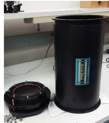
Fig. 7. Subsea housing from PREVCO™ that will be used to house the illuminator for tank testing. Its size was chosen to be compatible with the REMUS 600 AUV. Internal dimensions: 25 cm diameter x 45 cm long
