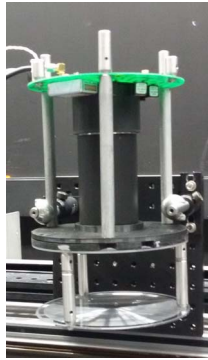
Fig. 8. Assembled receiver, showing the collection optics and PMT.
