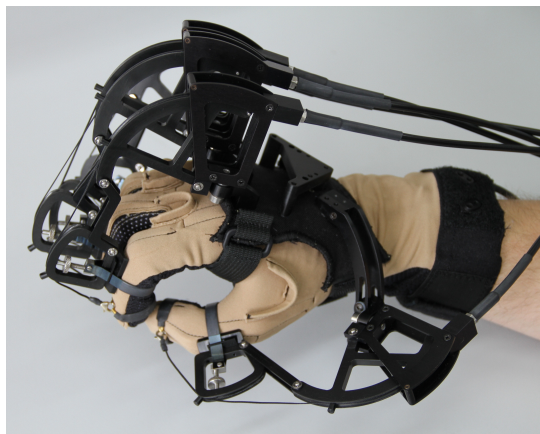
Fig. 13: Haptic feedback of grasped objects
