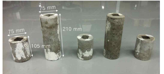
Fig. 5. The landmark consists of two large concrete columns (75 mm x 210 mm, D x H) and three small concrete columns (75 mm x 105 mm, D x H).
