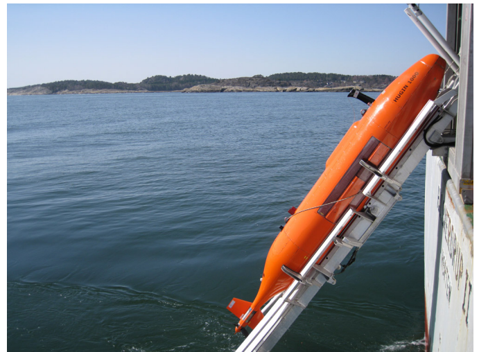
Fig. 1. The HUGIN autonomous underwater vehicle with the HISAS 1030 interferometric SAS during launch from HU Sverdrup II.
