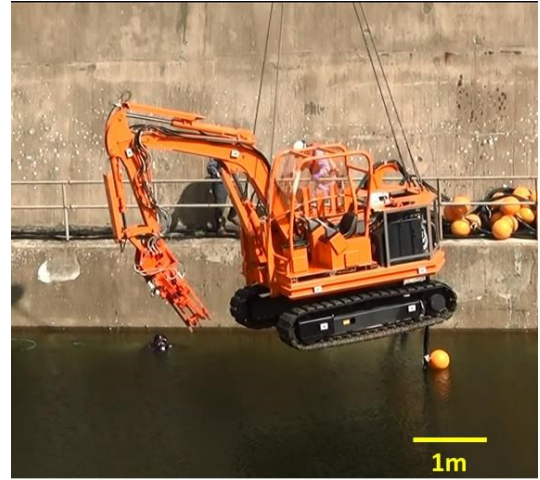
Figure. 3 The underwater teleoperated excavator (ROV-1).
