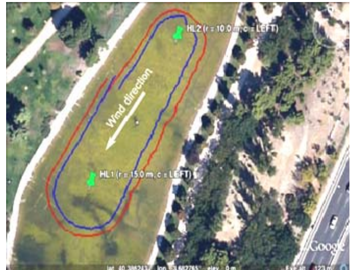
Figure 20. Experimental confirmation of boom towing with a parallel formation of USVs
