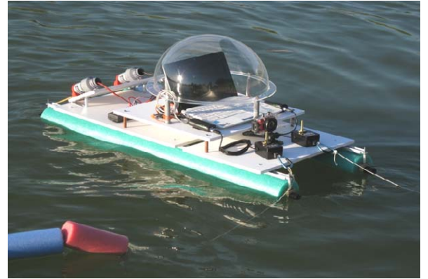
Figure 8. the data gathering floating platform.
