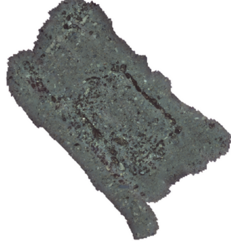
Fig. 2. High-resolution photo-mosaic map of a rectangular room reconstructed from stereo-vision imagery gathered during a survey of Pavlopetri, Greece in 2010.
