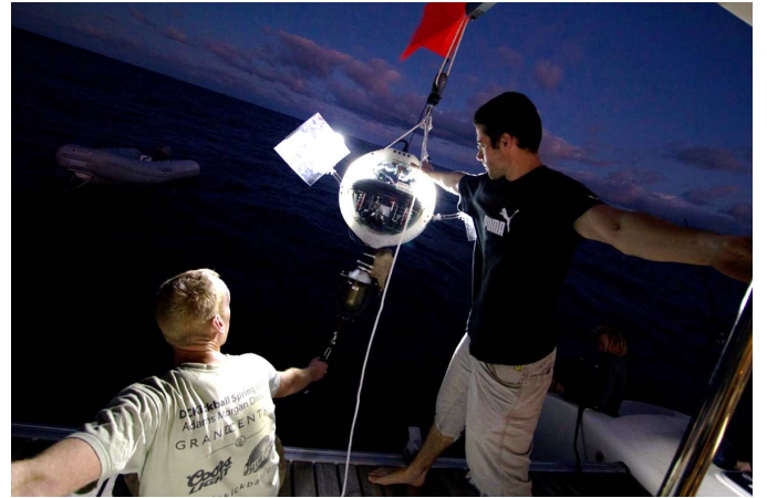
Fig. 5. National Geographic engineers prepare to deploy a Deep Ocean Dropcam into the Puerto Rico Trench. (photo courtesy of Shelbi Randenberg)
