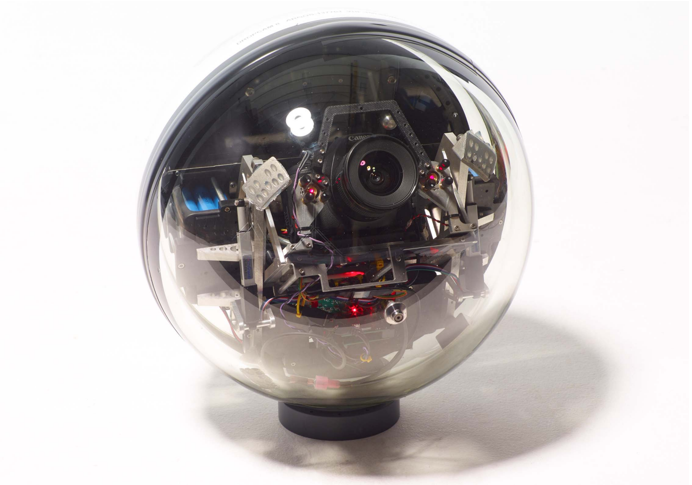
Fig. 3. View of the camera system mounted in the bottom hemisphere of the pressure housing (photo courtesy of Mark Thiessen and Rebecca Hale)
