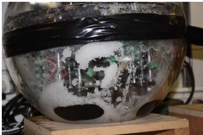
Fig. 8. Damaged DOD used with the BOBO lander. The bottom hemisphere is full of glass dust from internal spalling due to a catastrophic event.
