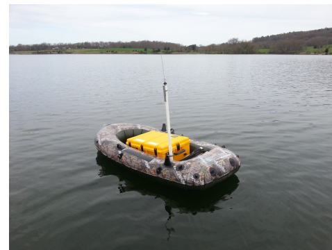
(b) Acoustic buoy deployed on a raft as part of a long baseline acoustic positioning and communication system
