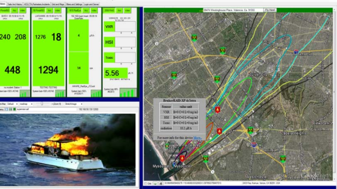
Fig. 9 LINCC Multi-Meter ICBRNE graphical user interface showing sensor instrument readouts, contextual video, vessel location and real time dispersal models in an integrated GIS environment
