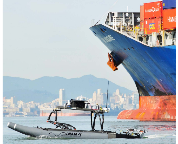
Fig. 2 The 16' Sentinel WAM-V conducting an automated harbor patrol
