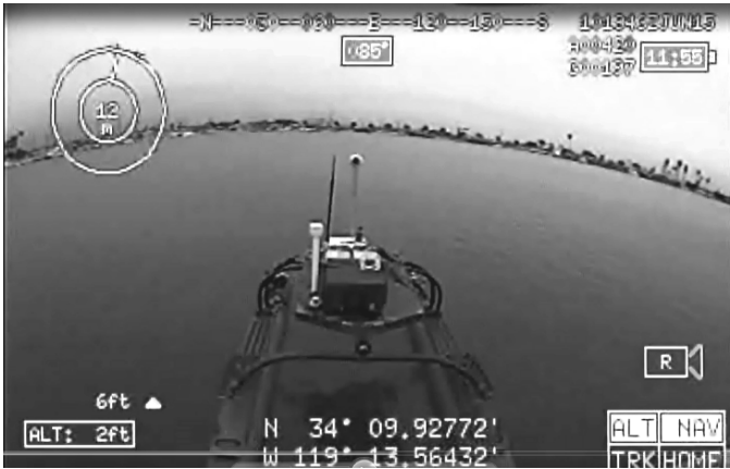
Fig. 7: Aerial drone video point of view during landing approach to the Sentinel WAM-V marine drone
