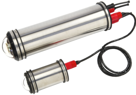
Figure 3. Optical modem, 4500 meter-rated. The receiver (top) and emitter (bottom) form one half of an optical modem system. This set was installed on Sentry , and a similar set was installed on the node. The receiver housing has a 6 inch outer diameter.
