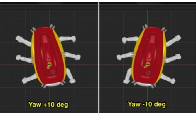
Fig. 14 Yawing motion fixing the six feet to extend viewing field
