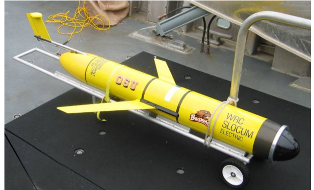
Fig. 1: A Slocum glider, used for long endurance environmental monitoring missions
