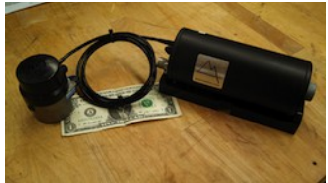
Figure 4: Tritech Micron mechanically scanned imaging sonar with Greensea embedded feature-based navigation system and MEMS-based INS.
