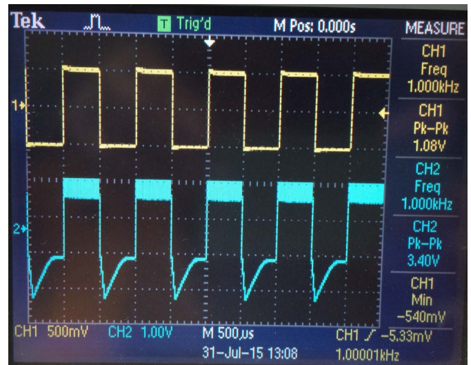
Figure 10: Scope capture of input of 1Vpp and V_g of the MOSFET. Yellow square wave on the top represents the input of 1Vpp. Blue waveform on the bottom represents the V_g of the MOSFET.
