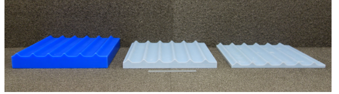
Fig. 3. Fabricated rippled samples used in this study. Machinable blue wax (left) shown with 3D printed (VeroBlue) samples with thick base (middle) and thin base (right). The length of the ruler in the foreground is 150 mm.
