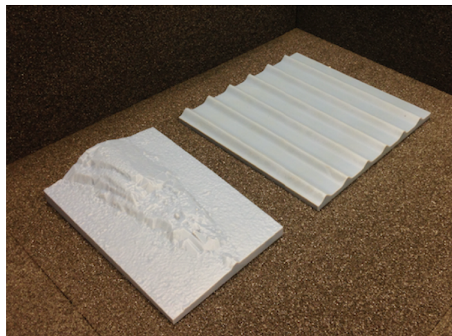
Fig. 1. Examples of 3D printed geometries. A 1/67 scale representation of a 15 m long rock outcrop from Larvik, Norway is in the foreground, and a rippled surface of 304 mm side length is in the background.
