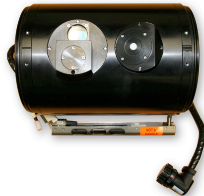
Figure 1: Fluorescence Induction and Relaxation (FIRe) sensor integrated into a Teledyne Webb Research Slocum Glider payload.
