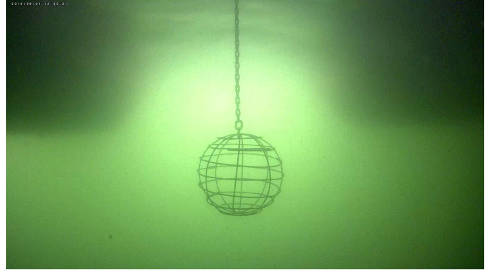
Fig. 2. Sample image of calibration target. Note strong backlighting and low water visibility. The dark shapes in the upper corners are the pontoon hulls of the test vessel.
