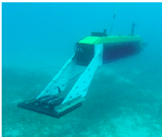
Figure 2 The Hybrid Autonomous Underwater Vehicle HAUV-1000 or "Dolores" is a hybrid AUV-ROV with highly accurate positioning and control realized through 1 fixed lateral thruster, 1 fixed vertical thruster, and 2 aft forward thrusters. The MFDA EM sensor array is shown here mounted from the bow and extending down and in front of the platform.
