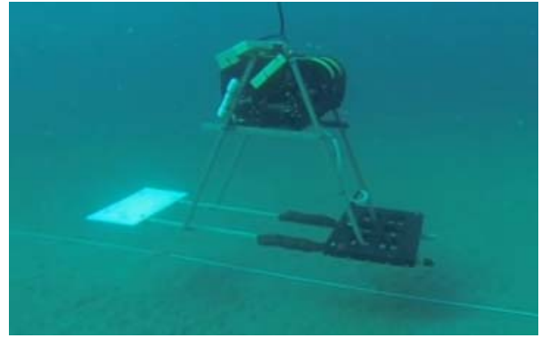
Figure 1. The integrated VLBV-EM system is based on the Seabotix LBV inspection class ROV system. The MFDA sensor array is mounted below and forward of the vehicle platform with a counterbalancing deflector below the stern to provide stability in turn and dive maneuvers.
