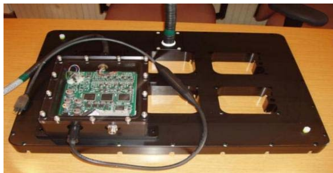
Figure 3. The Multi-Frequency Digital Array (MFDA) is a frequency-domain multi-sensor array capable of detecting and characterizing both ferrous and non-ferrous conductors on or below the seafloor. Originally developed for finding buried explosive hazards, this system was modified and retrofitted for marine EM deployment from ROV's by our team in 2011.
