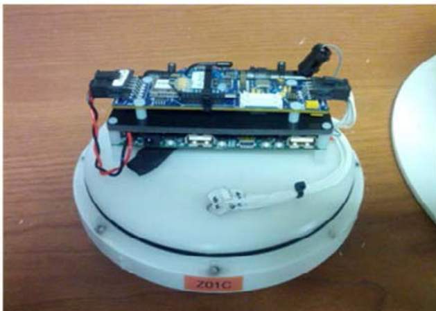
Fig. 4 Lower Camera Housing (contains the Smart Module, Linux Gumstix processor, and Wi-Fi transmitter with the power port at the bottom of the housing)
