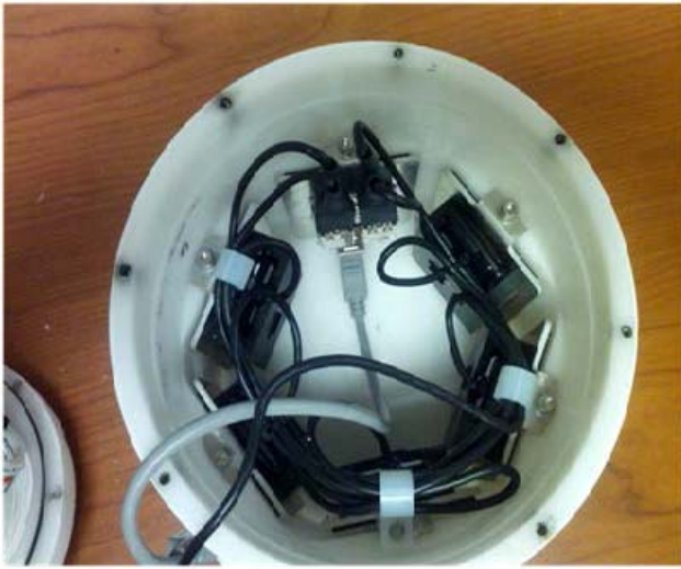
Fig. 3 Upper Camera Housing (contains five web cameras, a camera interface board, and cabling)
