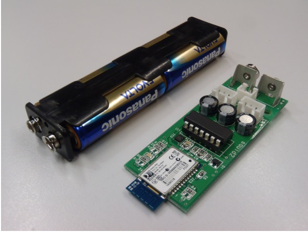
Fig. 3. Printed circuit board within ubiquitous sensor.
