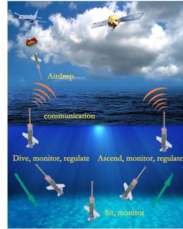
Fig. 2. the pneumatic-driven airdropped underwater profiler and moves towards the target bearing with hydrodynamic drive.
