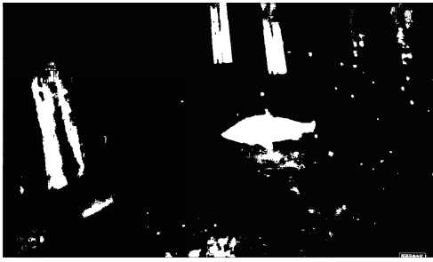
Fig. 4. Compare the current frame with the average background by background subtraction. The result indicates that the white pixels are possible moving object pixels. But due to the poor image quality and noise caused by non-static objects, these pixels may cause errors.
