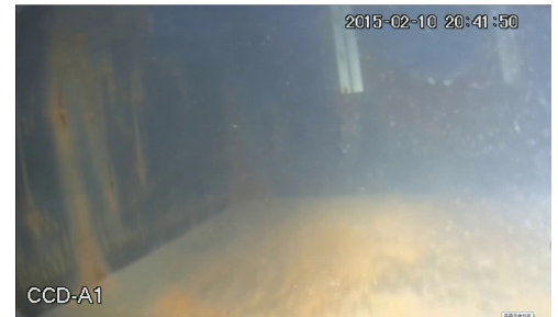
Fig. 3. Use 15 frames from the beginning of underwater video to establish an average background. There is no objects in the average background.
