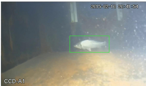
Fig. 7. Draw a green rectangle to label the moving object. From the figure, we can see that the fish, which is what we want to detect, is labeled exactly.
