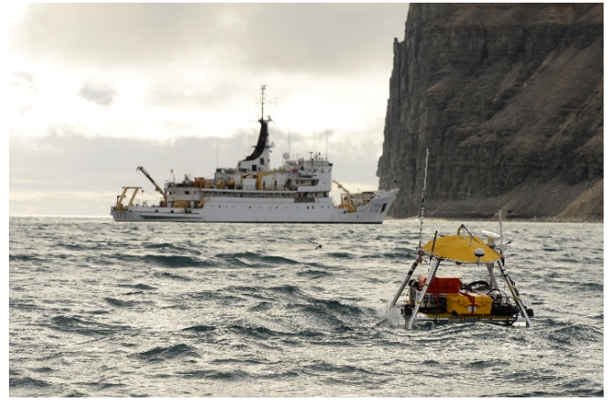
Fig. 5: USV-2600 sets up to run ahead of QUEST in a zig-zag pattern to survey water depths in-stride.
