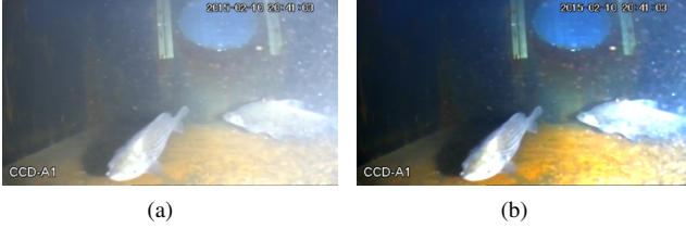
Fig. 2: “Haze” removal result. (a) input underwater image. (b) image after “haze” removal by dark channel prior.
