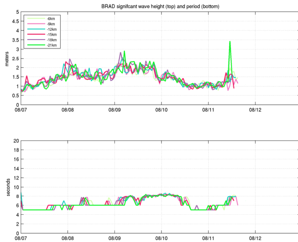
Figure 3: Wave estimates (top: wave height and bottom: wave period) from the BRAD 13 MHz site from August 7-13, 2015. The different colors represent the range cell of the wave measurement.
