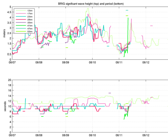
Figure 4: Wave estimates from the BRIG 5 MHz site, using enhanced blanking. Temporal coverage is improved relative to expected coverage based on the nearby LOVE site at the same time.
