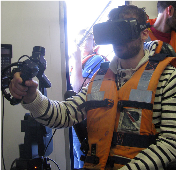
Fig. 9. The HMD allows the operator to have full control over the whole system, without having to rely on a second operator.
