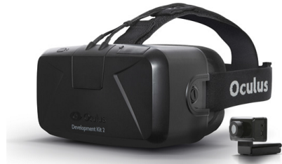
Fig. 3. The Oculus Rift is the HMD chosen for increasing the telepresence experience and to actively control the ROV 30k.
