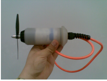
Fig. 10. Thruster of the ROV Version 1.0
