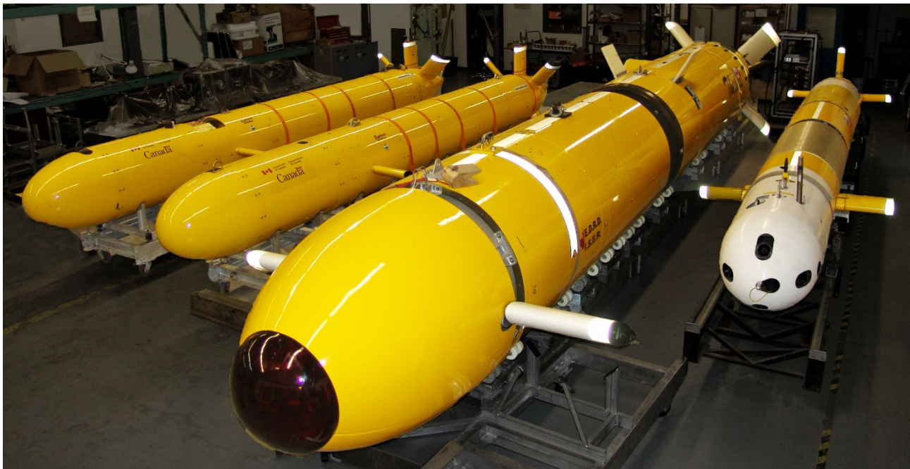
ISE's AUV Family of Vehicles (Two Arctic Explorers, THESEUS, ARCs)
