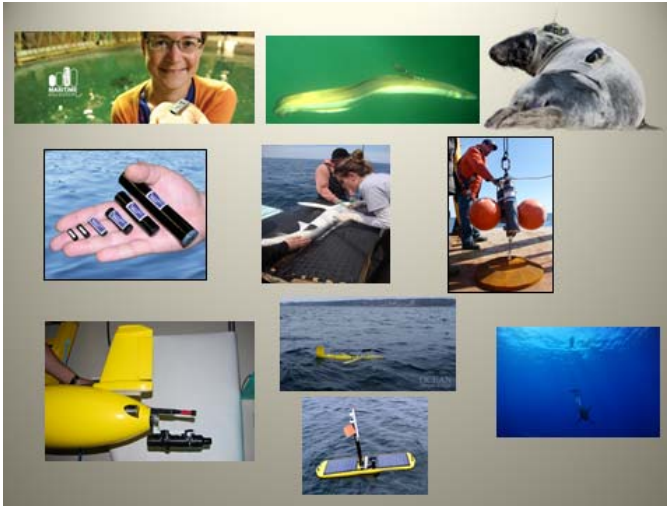
Fig. 1: Top (left to right), Maritime Biologgers accelerometer archival tag, an American eel fitted with a pop-up satellite tag, a grey seal bioprobe with a head mounted Argos satellite tag and a mobile acoustic receiver that transmits its data through the Argos tag via a Bluetooth connection. Middle (left to right): VEMCO acoustic tags, OTN researchers surgically implant an acoustic tag in the body cavity of a blue shark, deployment of a VR4 acoustic receiver unit equipped with an acoustic modem. Bottom, left-VEMCO VMT receiver mounted below the tail of a Slocum Glider; middle (upper),- Slocum glider; middle (lower)-surface float of the OTN Wave Glider; right-Wave Glider towfish containing the hydrophones to download VR4 receivers attached to the propulsion sled that converts wave energy to propulsion which in turn is tethered to the surface float
