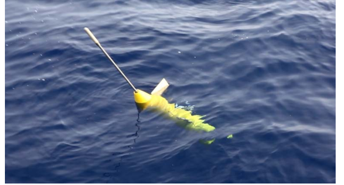
Fig. 4: A SeaWing Glider (1000m-class) which was developed by Shenyang Institute of Automation (SIA), Chinese Academy of Sciences.
