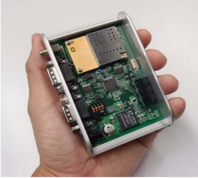
Fig 2. Picture of the microCube that are equipped in the fishing vessels to collect the real-time location and speed data.
