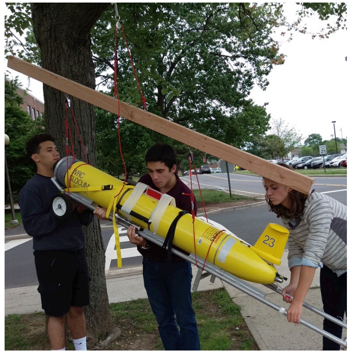
Fig. 4. The hanging apparatus allows the glider to freely move in 3D space with ease. Object such as a tree is required to hang the apparatus.
