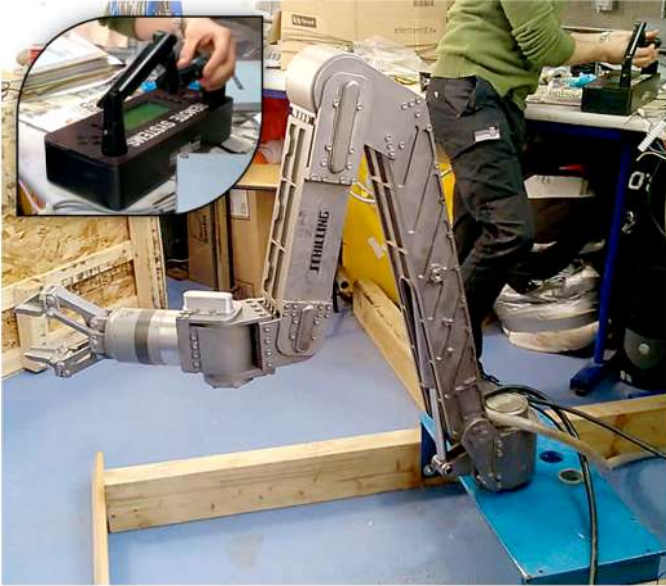
Fig. 3. Schilling Titan 2 - Hydraulic Seven Function Subsea Manipulator
