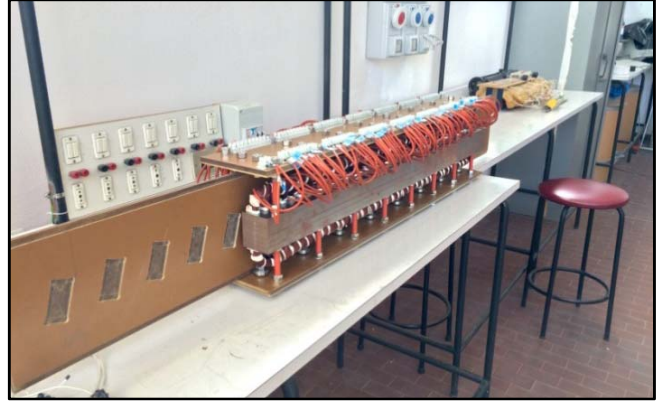
Fig.6 – The laboratory prototype of the Electric Generator
