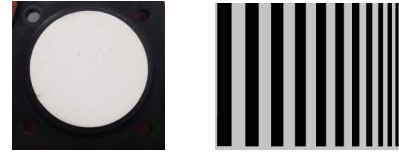
Figure 7: Spectralon medallion (left) and target for the four meter test.
