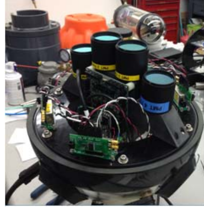
Figure 4: Open receiver housing showing the 4 collector assemblies (PMTs).
