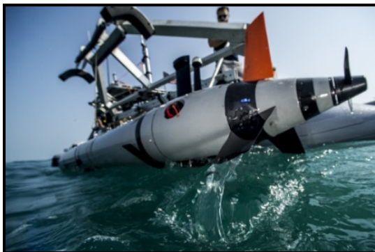
Figure 4: A MK-18 MOD 2 Kingfish Unmanned Underwater Vehicle, is recovered aboard a Rigid Hull Inflatable Boat (RHIB) in the 5th Fleet area of responsibility. (U.S. Navy photo by Mass Communication Specialist 1st Class Blake Midnight/Released)
