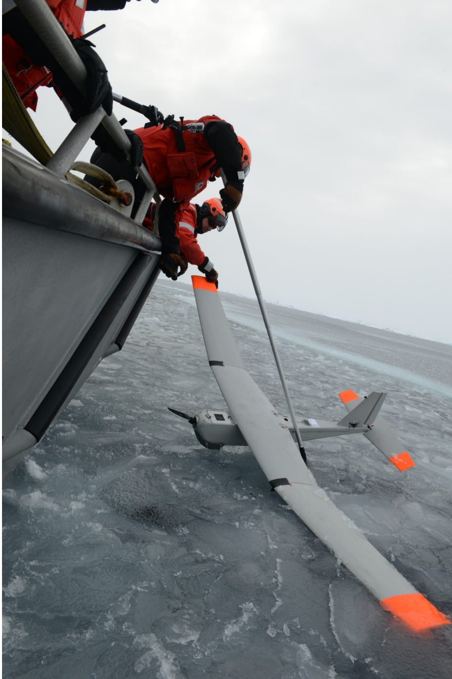
FIGURE 2: Unmanned Aerial Systems – A NOAA Puma AE is being recovered from the ice during Arctic Technology Evaluation 2013 testing in the Chukchi Sea. (USCG Photo by Petty Officer 2nd Class Grant Devuyst.)
