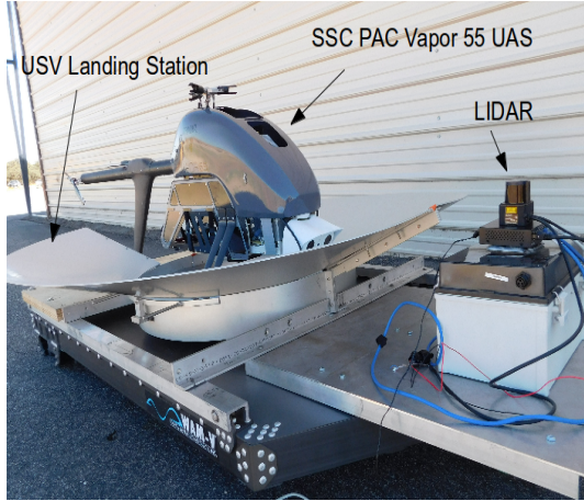
Figure 3: Modified (payload module added) UAS locked onto the LIDAR equipped landing station
