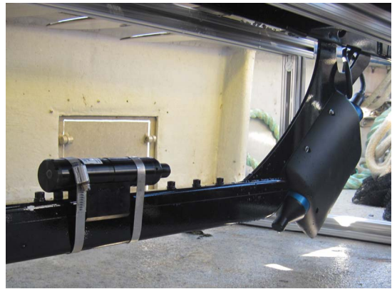
Figure 1: VEMCO VR2C and VMT installed on Wave Glider SV2
