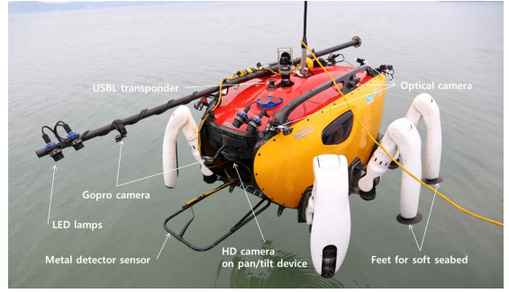
Fig. 3. The Crabster CR200 with metal detector.
