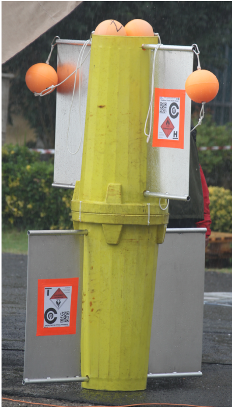
Fig. 4. A double-height underwater mapping fiducial with plastic cylinders and aluminum wings.
