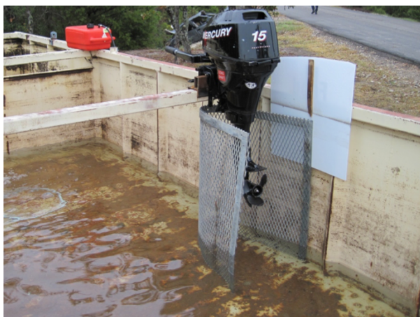
Fig. 23. An outboard boat engine mounted inside a shallow water tank to generate current.
