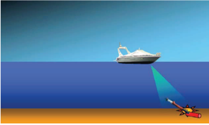
Fig. 3. A non-disposable ASV guides a disposable neutralization AUV.
