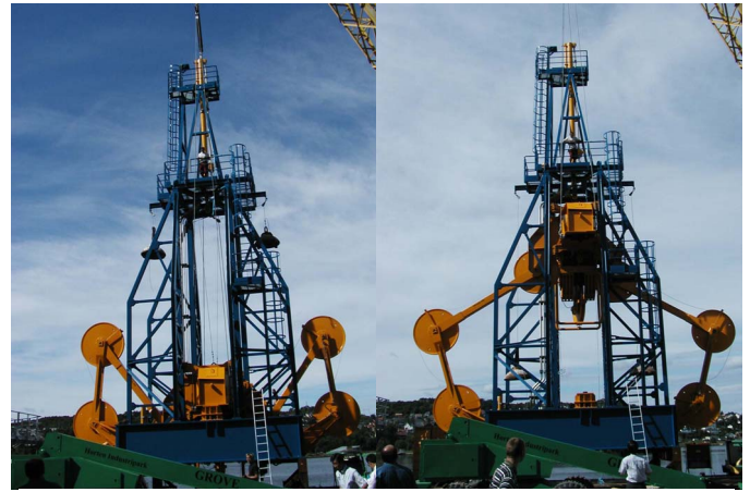
Fig. 3 Sheaves at the Top of the Derrick Left: Fixed Sheave Block is at the lowest position Right: Fixed Sheave Block is at the highest position
