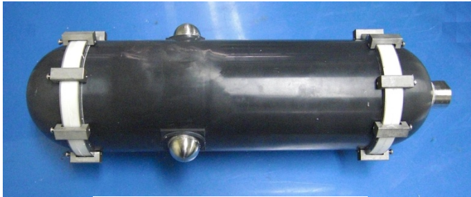
Fig. 5 Scale Model Pressure Vessel Cylinder Length : 252mm Inside Diameter: 90mm
