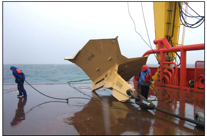
Figure 2. Drag-installed Vertically Loaded Anchor
