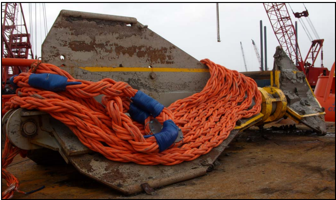
Figure 6. OMNI-Max Upper and Lower Fluke Fins Size Difference
