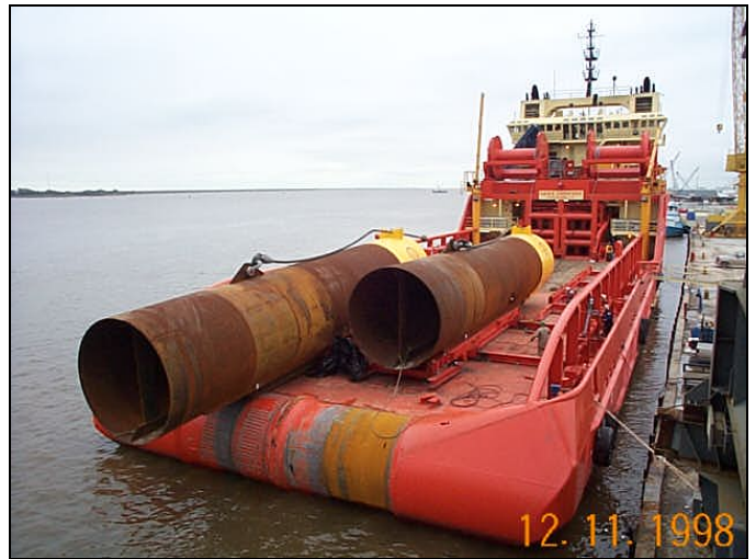
Figure 3. Suction Pile Anchors
