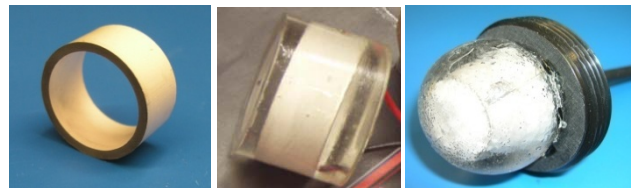
Figure 2. From left to right: The raw piezoelectric ring ceramic, the potted ceramic, the transducer in the potting compound mounted to a prototype plate to be attached to a modem housing.
