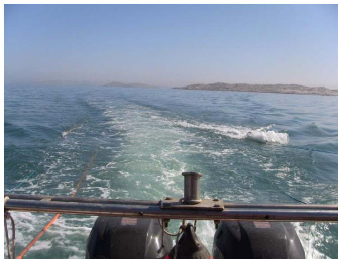
Figure 6. Deployment of the ARS (orange cable) in conjunction with a Boomer system (blue cables either side of the vessel wake).
