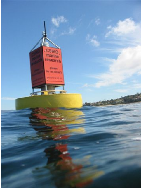
Fig. 1: Fixed node at the surface, used to acoustically communicate with underwater sensors (Fig 2.) and wirelessly with the CSIRO station.
