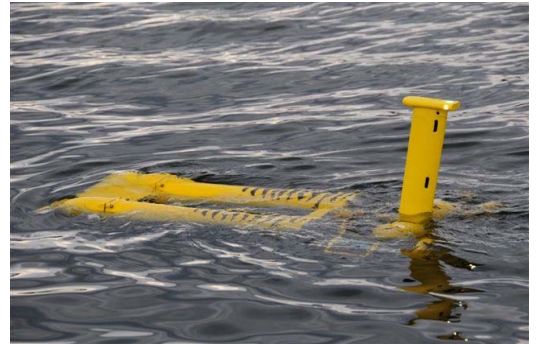
Fig. 3: The mobile node (AUV) developed at CSIRO where sensors are installed to collect data between the fixed nodes. This AUV is 1.2-m long and is able to navigate up to 50-km a day and up to 100-m depth.
