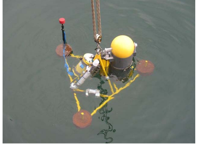
Fig. 2: Fixed riverbed node being deployed in the Derwent estuary, Tasmania, Australia.
